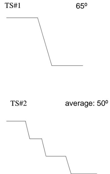
Figure 1. Sections corresponding to Test Site #1 (top) and Test Site #2 (bottom). Each bench is approximately 12-13m high.
