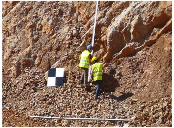
Figure 4. Targets and surveying rods were deployed around the scene for georeferencing.
