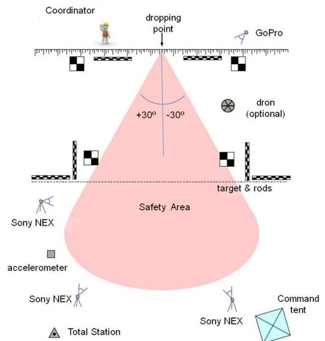
Figure 2. TS#1. Plan view with the planned equipment and personnel layout.
